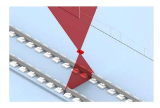
The OPTIMESS CSD, on the other hand, is ideally suited for the simultaneous detection of the contact wire and the rails. This eliminates the need for compensation. A calibration is also not necessary. This makes it ideal for simple, accurate and reliable measurement of contact wire height and lateral position.
